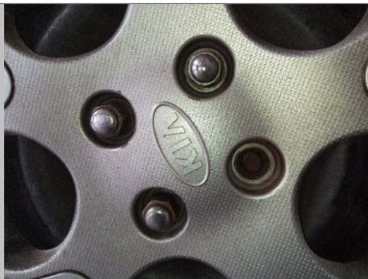
RIGHT FRONT WHEEL STUD DAMAGED
