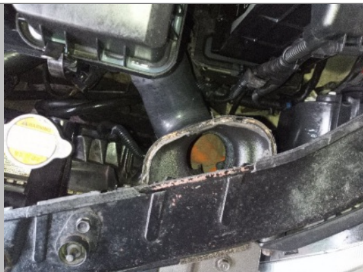
AIR INDUCTION PIPE HOUSING MIS
