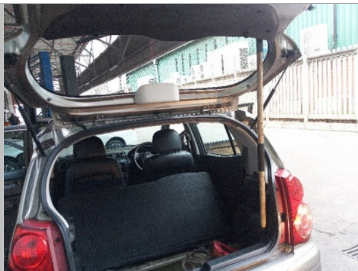
TAILGATE SHOCKS DEFECTIVE
